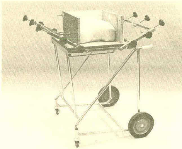
Fig. 2 Foam-in-Box equipment ready for pouring foam.
