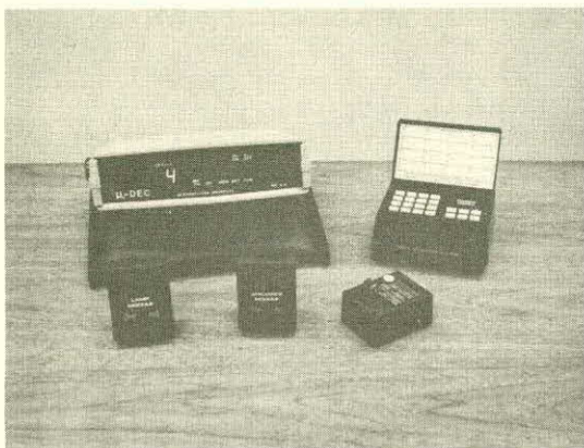
Fig. 1 MicroDEC control unit, BSR receiver modules and BSR system command console.
