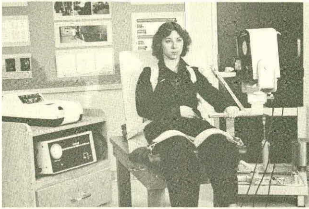
Fig. 9. Modified Cybex equipment to measure shoulder isokinetic strength.
