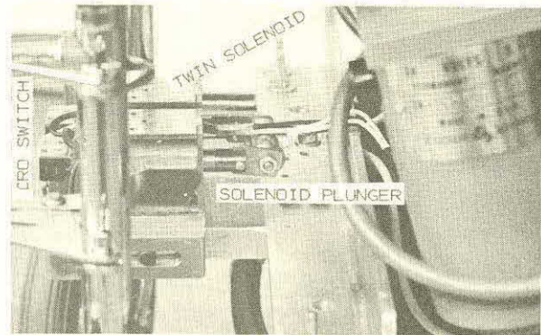
Figure 4: Twin solenoid assembly showing position of microswitch and solenoid plunger. After brakes are applied, high power coil is disconnected and low current drain coil is connected to hold brakes in position.
