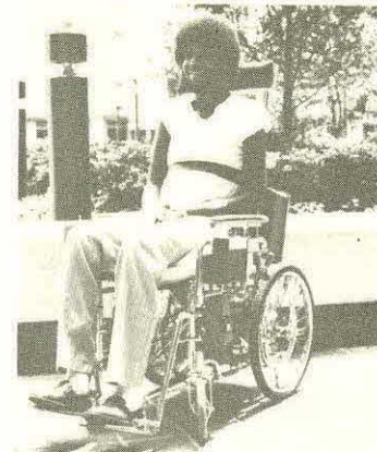
Figure 4. Application of the shoulder position controller for control of a powered wheelchair.
