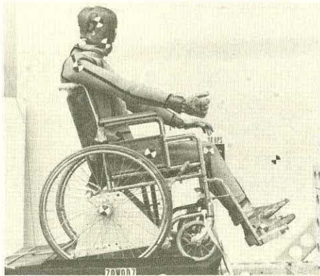
Figure 6. Sled test set up for CCI platform with 165 lb. restrained by lap belt
