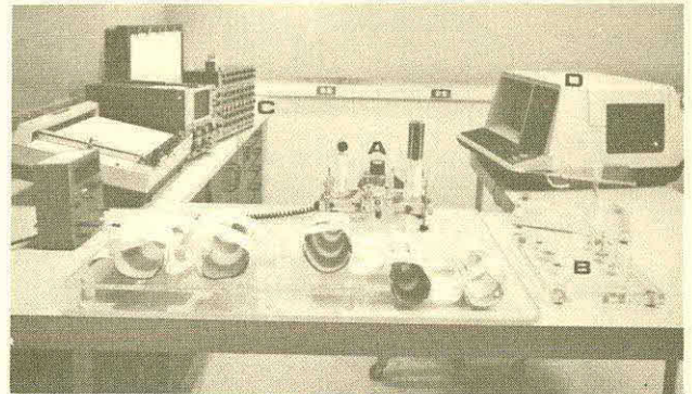
Fig. 1. Hand evaluation equipment: (A) Strength meters, (B) Peg board, (C) EMG amplifier, (D) Computer terminal for data retrieval and analysis.
